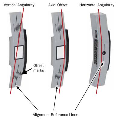
For different pulley edge thicknesses, use the offset marks on the face of the reflector to establish the amount of offset. The marks are in 1/8-inch increments.
