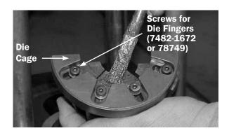
**4.** Periodically check bottom of die cage and top surface of die back up ring for cleanliness.
