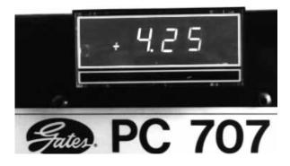
11. Turn knob to a setting below the desired setting. Then turn knob back up to the desired setting. (Digital readout numbers may jump a number, e.g., 5.50 to 5.49 or 5.51. This will not affect crimp diameter of the coupling.)
