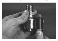
**3.** Place a visible mark on hose cover at the insertion length shown in the crimp data manual or use MegaCrimp Insertion Tool (7482-1342).
