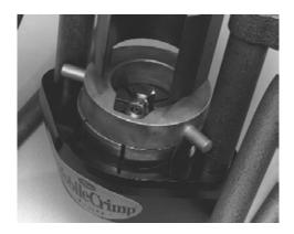
6. SWING CYLINDER INTO CRIMPING POSITION Using the handle, swing cylinder toward you and lock into place with lock pin.
