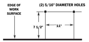
Drill two 5/16" diameter holes then use mountig holes or clamps to fasten stand to work surface.
