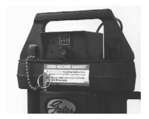
Turn pump on by pressing and holding the power "on" switch, (see pump operating manual for switc location) which extends the ram.
