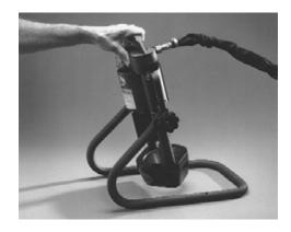
Turn the knob on the controller to a setting of **400**, which allows the ram to extend approximately 1".
