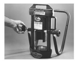
Slide the two halves of the stand together and attach to the crimper at the pivot bolts.
