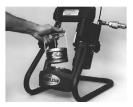
Apply a thin layer of Molykote lube to the top of the die set.
