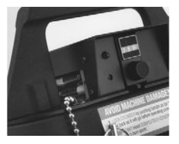
Replace the batteries and position as shown on holder. Replace and secure the side cover.
