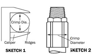
Measure halfway down the crimped portion of the ferrule (Sketch 2).
