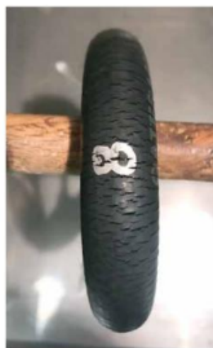
Figure 3: Cover cracks caused by ozone.
