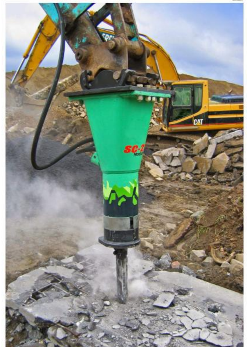
Montabert recommends every 40 to 50 hours of breaker operation to remove the tool and inspect. Reseal the breaker anywhere from 350 to 500 hours if the hammer is not leaking.
