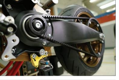
Fig. 3: Narrow, lightweight drives improve performance on an e-motorcycle.
