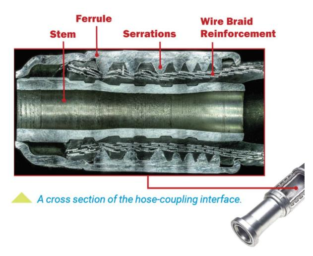
Once the correct coupling components are chosen to be qualified with a specific hose, the next step in qualification is to develop a manufacturer-provided crimp specification. This specification often refers to the final crimped OD of the coupling ferrule after it has been attached to a specific hose, measured using calipers on the flat portions across the ferrule diameter. To develop these crimp specifications, coupling development engineers estimate
