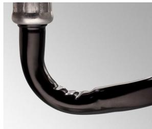
Inferior bend reduces coolant flow.
