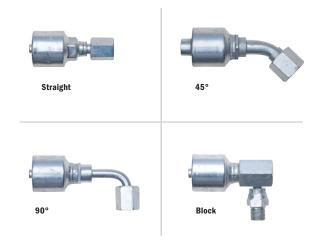
Hose ends and thread ends are measured by industry standard dash sizes. The hose end dash size refers to the inside diameter in 1/16" (except for PolarSeal® hose, SAE 100R5 and SAE 100R14 which are based on tube 0.D. and are smaller than the dash size implies), e.g., -8C5C hose is actually 13/32" I.D.
