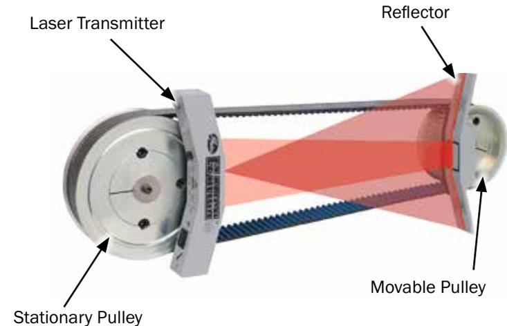
The following diagrams depict misalignment conditions using the Gates EZ Align™ and the corresponding corrections as observed on the units.
