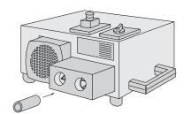
5. Slide the screw connection parts over the end of the pipe as illustrated.
