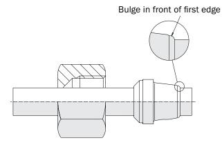
10. After it has been tightened, loosen the connection again; check whether the space before the edge is filled out. The ring may turn.
