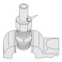
8. A marking applied to the union nut with a pen makes it easer to determine whether the prescribed turn has been carried out.
