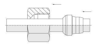
5. The shoulder of the cutting ring must be facing the union nut.
