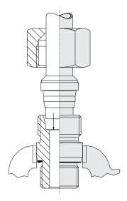
7. Then tighten the union nut until the tube cannot be turned anymore in the screw connection – the cutting ring is clamped onto the tube.
