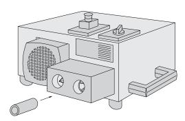
4. Push screw connection parts over the pipe end as illustrated.
