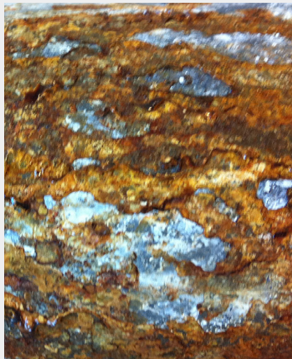
CLOSEUP OF OE STEEL TUBE AFTER A 400 HR SALT SPRAY TEST
