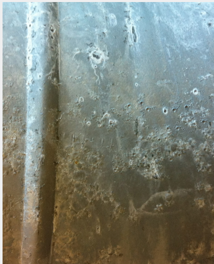
CLOSEUP OF GATES STEEL TUBE AFTER A 400 HR SALT SPRAY TEST
