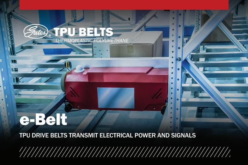
Our advancements and expertise in material science, design engineering, and processing technologies allow Gates to develop TPU belts that can transmit electric power or signals while incorporating the high tensile strength of the steel reinforcement. The steel cords are exposed at the belt ends for electrical connector attachment. The openended e-Belts can be cut to custom length. Several timing belt pitches and flat belts are available.
