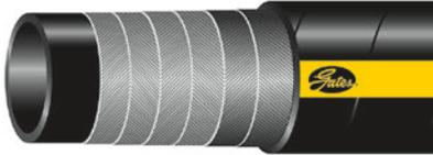
**Spiraled reinforcement** on hydraulic hose is typically wire or textile and has four or six layers (plies). Spiral-reinforced hose can typically handle more severe applications with longer impulse service life.
