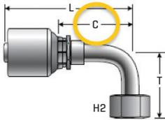
Cut-off value “C” is the length of that part of the coupling not directly in contact with or applied to the hose. Therefore, subtract the two “C” values from the total length of the assembly and you will have the approximate hose length to be replaced.
