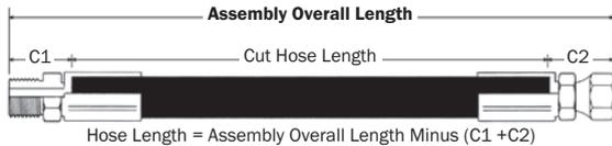
SAE Length Tolerances for Hydraulic Hose Assemblies and Specified Hose Lengths (Reprinted from National Hose Assemblies Manufacturers Association NHAM-STD-2)
