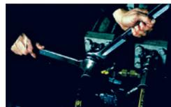
5. Thread the other end of the assembly, taking care not to twist the hose. Use a wrench on the fitting's backup hex while tightening.
