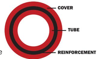
The tube is the part of the hose that comes in contact with the hydraulic fluid. Reinforcement allows the hose to withstand internal pressures, or in the case of suction/ vacuum hose, external pressures. Hoses generally have braided, spiraled or helical reinforcement. The type of reinforcement depends on the intended use of the hose.
