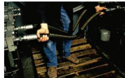
3. Lay the hose assembly into the routing position to verify length and correct routing.
