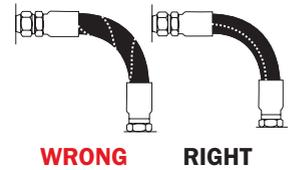
5. Avoid twisting of hose lines bent in two planes by clamping hose at change of plane.
