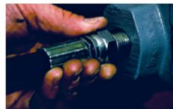
4. Thread one end of the assembly onto the port or adapter. Install angled fitting first to ensure proper positioning.
