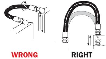
4. When installing hose, make sure it is not twisted. Pressure applied to a twisted hose can result in hose failure or loosening of connections.
