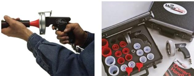
Gates MegaClean™ system uses shop air and projectile to sweep through the inside of the hose for improved cleanliness. Pressurized launchers and compatible nozzles blow foam projectiles through the inside surface of the hose, sweeping away fine particles of loose dirt and contaminants. The projectiles are 20–30 percent larger than the hose I.D., and leave nothing behind but a clean hose.
