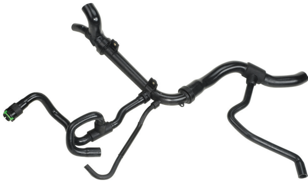
Coolant hoses have become increasingly complex with multiple branches and connections.
