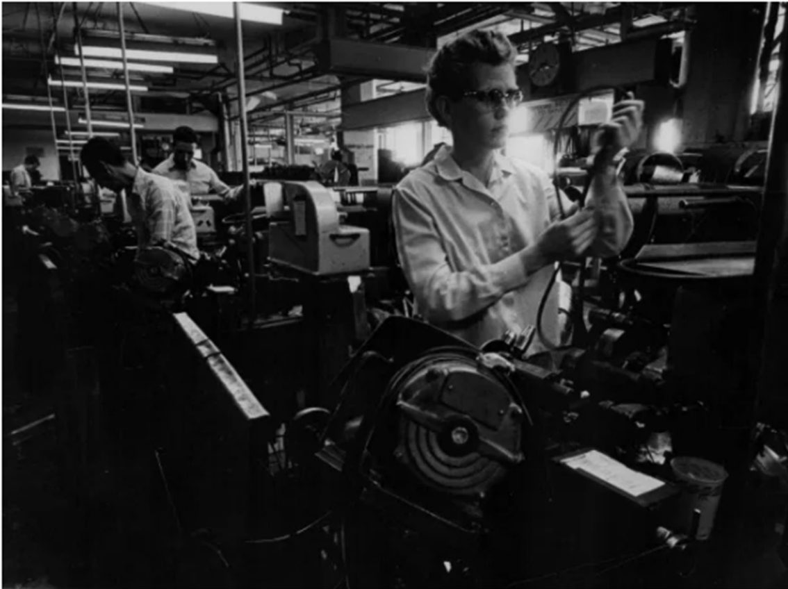
Duane Howell, The Denver Post A characteristic V-shape is cut into Gates belts by skiver operator Shirley Sturtheit at Gates Rubber Company on Nov. 3, 1965.
