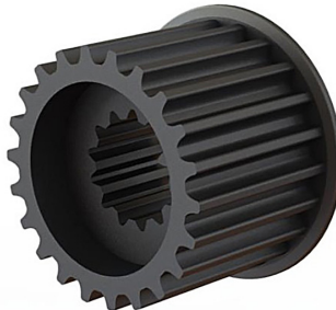
8M-22T, 41mm wide, 1 flange, 13Z spline
