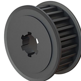
8M-25T, 20mm belt, 2 flange, 6T straight spline
