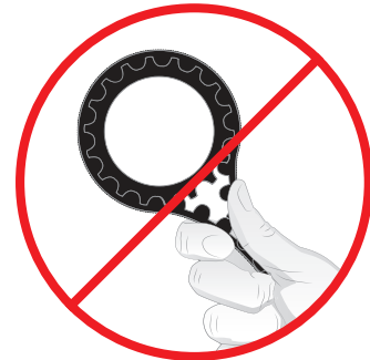
DO NOT USE BELT AS A SPROCKET REMOVAL TOOL
