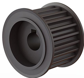
8M-22T, 41mm wide, 2 flange, keyway
