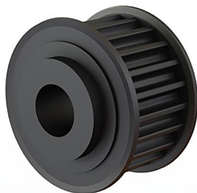
8M-25T, 25mm belt, 2 flange, plain bore
