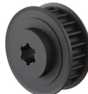
11M-22T, 20mm belt, 2 flange, 6T straight spline
