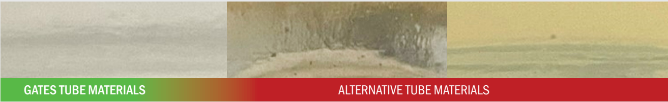
PG25 COOLANT AFTER EXTRACTABLES TESTING WITH VARIOUS DATA CENTER HOSES AT 80°C FOR 600 HOURS
