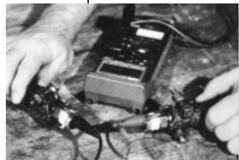
Hose assembly being tested with voltmeter.
