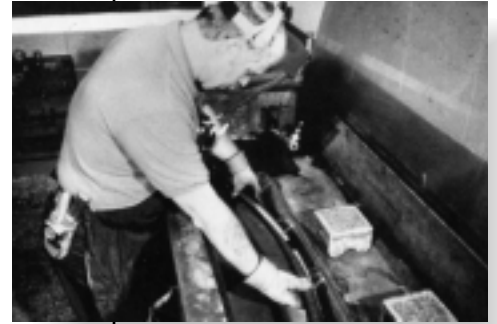
Hydrostatic hose testing.
