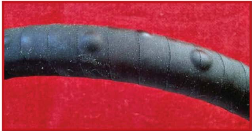
Blistering occurs when a hose is incompatible with the fluids that flow through it.
