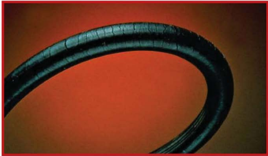
A hose with too small an inside diameter could generate unwanted turbulence in the fluid, which may cause the hose to crack.
